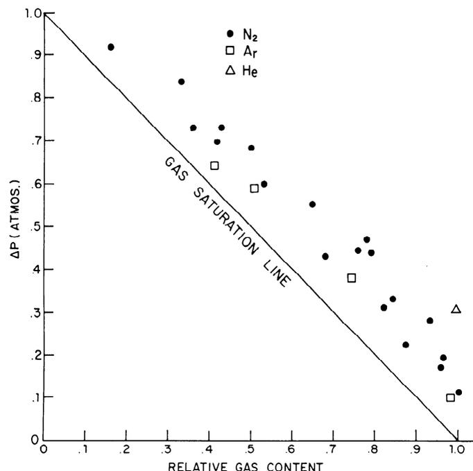
FIG. 2. Decompression required for bubble formation and growth in olive oil at various gas concentrations. Each point represents the midpoint of 40-torr pressure excursion between bubbles and no bubbles.
