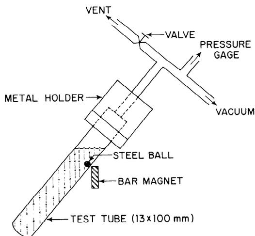
FIG. 1. Test apparatus for observing effects of viscosity and velocity.
