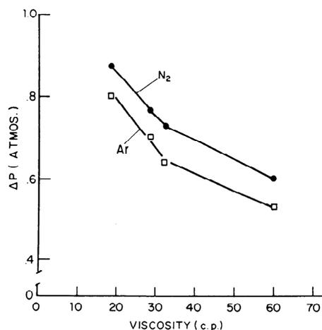
FIG. 3. Decompression required for bubble formation and growth in gas saturated glycerol-water solutions of various viscosities. Each point represents the midpoint of 40-torr pressure excursion between bubbles and no bubbles.
